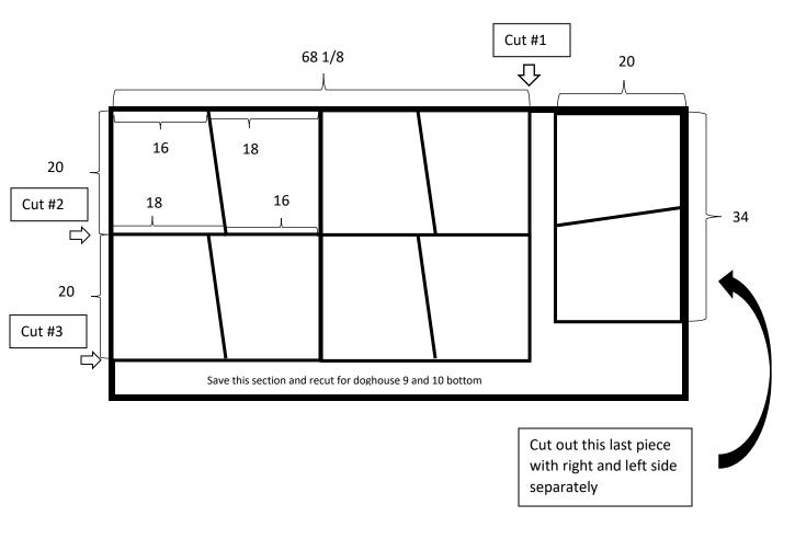
Once each of the 34 X 20 pieces are cut out from the sheet of plywood, mark the dividing line at 16 and 18 inches on opposite sides. Draw a line from each mark and then cut the diagonal line using a skill saw, or jig saw.
