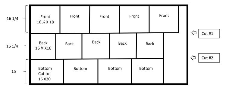
Cut the board lengthwise first to separate the fronts, backs, and bottoms. Then cut each strip to length as per measurements provided on the drawing above. Be sure that the bottom is 15 inches wide to ensure backs and fronts fit accurately.
